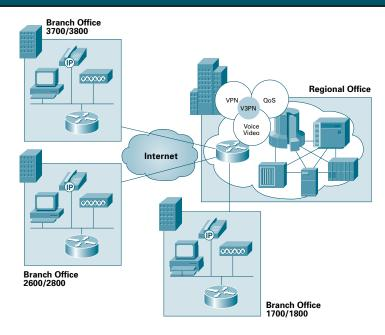
The figure above shows the Cisco 3800 Series routers converge voice, video, and data across a secure IPSec VPN network with high-quality, reliable performance. DMVPN creates tunnels on-the-fly based on user traffic. V3PN functionality provides QoS, multiprotocol, ease of provisioning, and secure connectivity.
